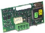
Fig. 5: Serial card for connection to a building management system or for master/slave control
